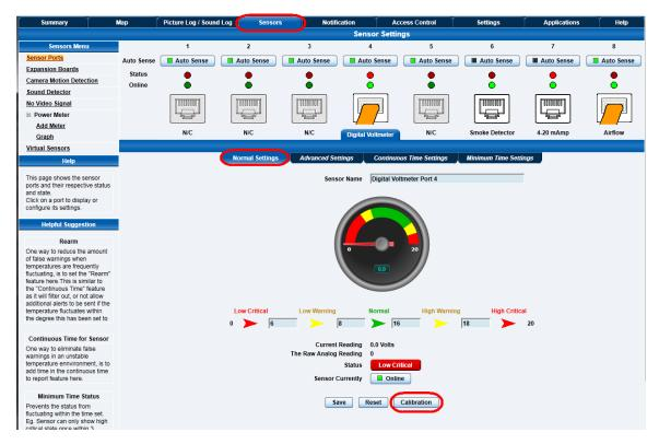
To calibrate the sensor, you would first disconnect the extension cable and connect the yellow calibration cable following the labels indicating which end is connected to either the base units RJ-45 port or the sensor connection. Now connect the green connector to the DC Input Voltage connector. Now as shown in the screen shot above you would log in to the base unit as an administrator, then navigate to the Sensors page >> Normal Settings, then click on the Calibration button.
