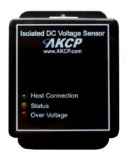
**Host Connection LED** = LED will be GREEN when connected successfully to your base unit. **Status LED** = LED will be blinking YELLOW when in an alert state. **Over Voltage LED** = LED will be solid RED if over voltage is connected to the sensor.
